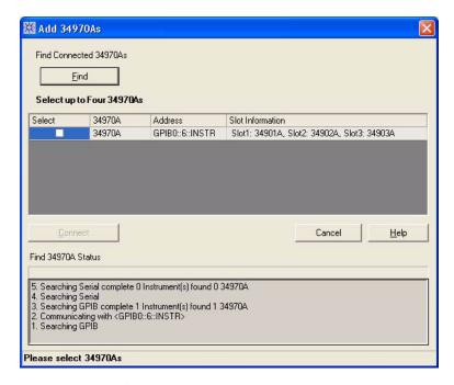
The **Find 34970A Status** area shows the status of the find operation. If you do not see any 34970As listed, check that the interface is connected and the 34970A is powered-on. For more information on troubleshooting configuration problems, refer to the Agilent Connection Expert application on the Automation-Ready CD ROM included with the 34970A.
