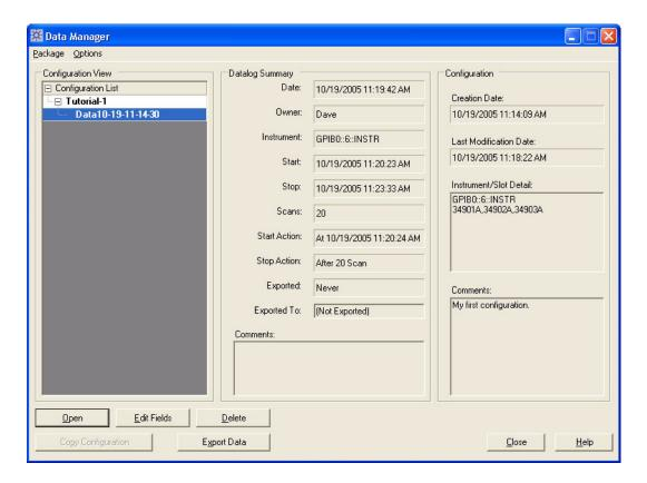
2 The Tutorial-1 configuration and the recently scanned datalog should appear in the Configuration View column. With the datalog selected as shown above, click the Export Data button. The Export Data dialog box appears and allows you to specify how to export the data and which data to export. For this tutorial, we will use the default export settings which creates a CSV (Comma Separated Values) file.
